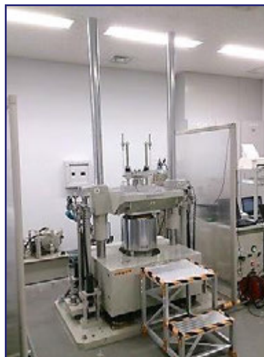
Board Drop Tester: Shinei Technology Model ASQ-700 (owned by Gunma Industrial Technology Center)
